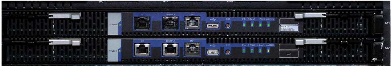
Figure 16: SX65xx with Dual Management Modules
